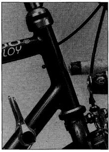
Goose bump: The pimple of a tire pump mount looks like an ugly blemish until you need to use it. Small features and concern for detail are much appreciated. Speaking of blemishes, there are none on this beautifully brazed Nobilette-constructed frame.
