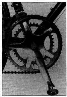
Ankle biter: Our Curve bike came set up with a Mavic gruppo. The French cranks are sleek-looking, but need to be slimmed down. Every RBA test rider complained of annoying ankle rub on the center of the units, even with the forgiving Speedplay pedals installed.
